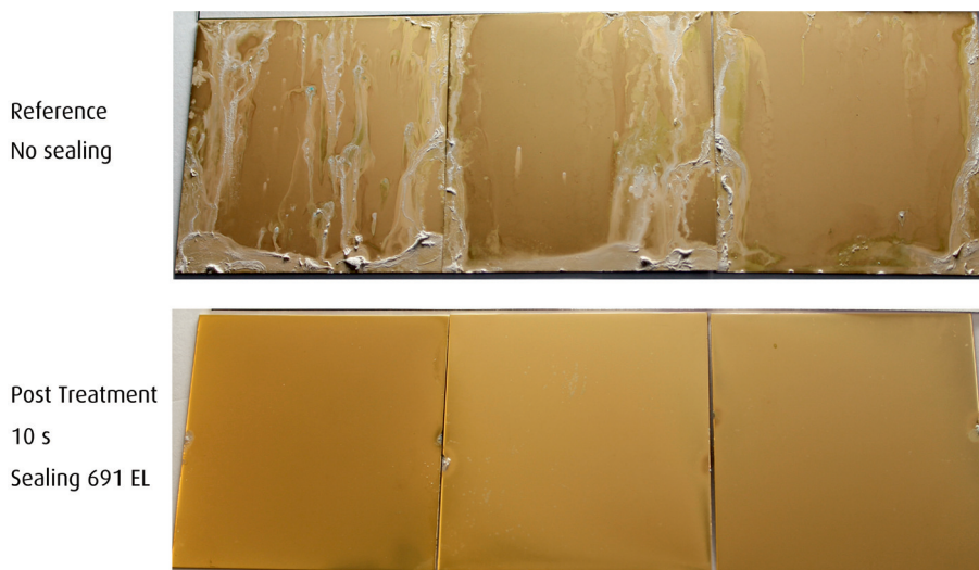
Fig. 9: Treated gold samples (0,4 \mu\text{m} ) demonstrate the strong protection level during the NSS test
